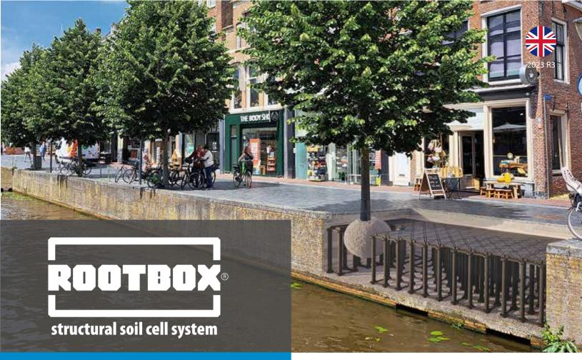
For climate adaptive cities we need big trees. Large trees have large roots. The RootBox offers enough unobstructed soil volume underneath roads, preventing roots to damage the pavement. The soil inside the RootBox is acting like a sponge but not only capturing and infiltrating water but also breaking down pollutions.
